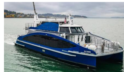
Sea Change, Switch maritime. 360 kW fuel cell, 242 kg, 250 bar.
