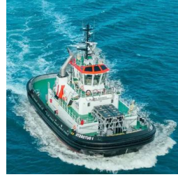
Hydrotug 1, CMB.TECH. 2 MW Engine. 400 kg hydrogen.
