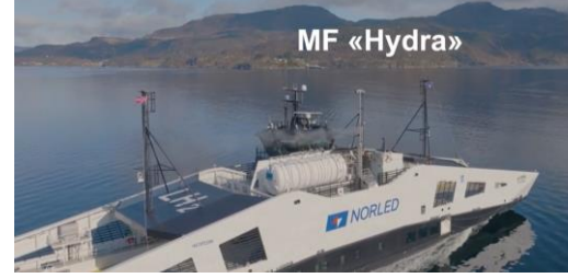
MF Hydra, Norled. Liquid Hydrogen (4T, 56 m 3 ). 2x200 kW fuel cell.
