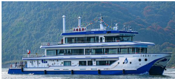
San Xia Qing Zhou 1 Hao (Three Gorges Hydrogen Boat 1), China Yangtze Power. 500 kW Fuel cell.
