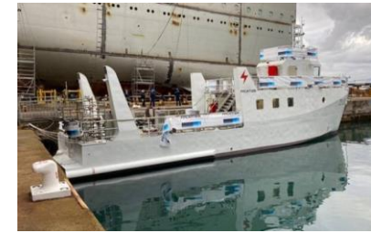
Zeus, Fincantieri 144 kW Fuel Cell, 50 kg hydrogen
